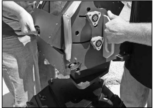
Fig. 22: Lift and place the MAX-Wedge on to the fully extended tripod.
