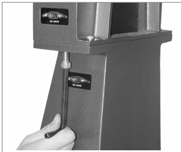
Fig. 15: Tighten the fork arm assembly using the provided hex key.
