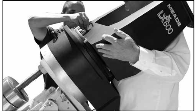
Fig. 32: Lift base, slide adapter into receiver and guide.
