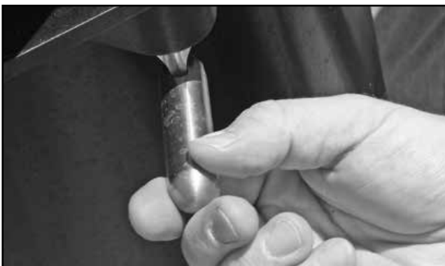
Fig. 10: Secure the drive base to the tripod by tightening the lever.
