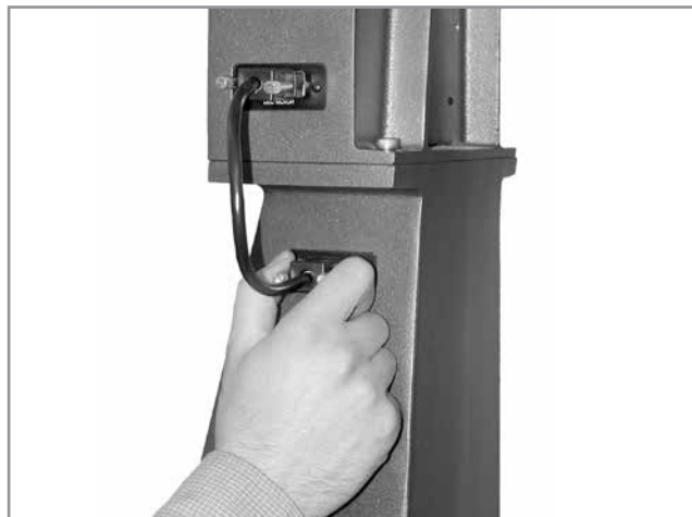
Fig. 16: Plug in the DB-9 connectors to provide power from the Dec. motor to the fork arms.
