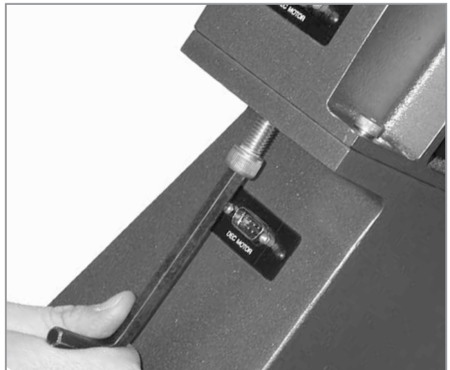
Fig. 36: Tighten the fork arm assembly using the provided hex key.
