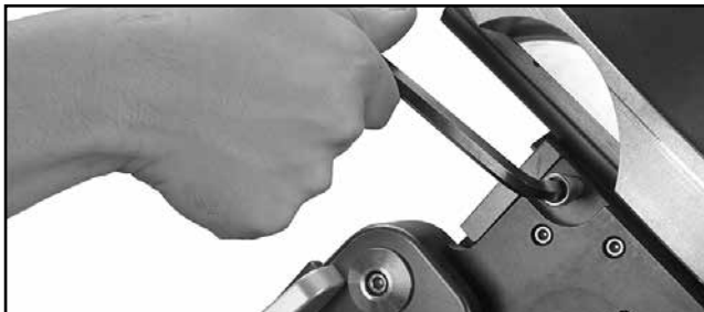
Fig. 31: Tighten the locking bolts.
